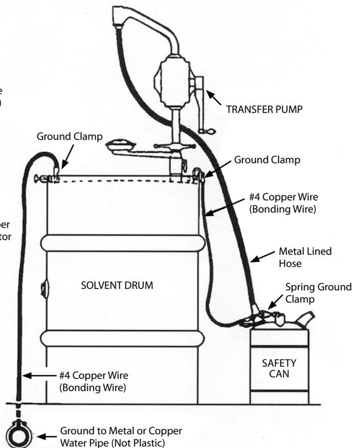
Two illustrations show grounding of solvent drums and methods of bonding drums to small containers being filled. If a good electrical connection is known to exist from the drum to the can through a metal lining and nozzle of the hose, the bonding cable between the drum and the container is not needed.
